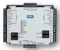
IDCUBE's ICAERO-X100 is the next generation access reader interface panel featuring door/ reader interface module supporting up to 2 doors, and an open architecture access reader & I/O interface platform that runs on embedded Linux, seamlessly integrates with "Access360" application. The ICAERO-X100 access control interface panel comprises of HID's Networked reader interface Aero X100 along with optional accessories, i.e., UL certified power supply, charging circuit, battery, and tamper switch.
