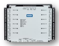
IDCUBE's ICAERO-X300 is an Output Control Interface Panel which supports 12 general purpose outputs as Form C relay contacts and 5 general purpose input circuits (supervised or unsupervised). The output interface panel comprises of HID's output interface module AERO X300 along with optional accessories, i.e., UL certified power supply, charging circuit, battery, and tamper switch. The ICAERO-X300 connects to the ICAERO-X1100 (master controller panel) through a high-speed RS-485 network.
